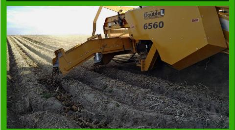
A RiteDrop sensor system on a Double L 6560 Windrower to keep the extended rear-cross stinger at the correct height.
