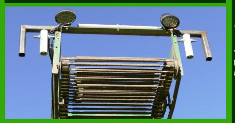
Conveyor height control on root crop and vegetable harvesters as well as on storage equipment, is still mostly a manual job for the operator. Operators must constantly watch the drop height and manually adjust the conveyor height to minimize the drop and so minimize bruise damage. This is fatiguing and stressful and sometimes hard to learn for an inexperienced operator.
