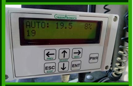
Controller with sealed keypad and display to engage & disengage automatic mode and to navigate the menu system for set-up and diagnostics.
